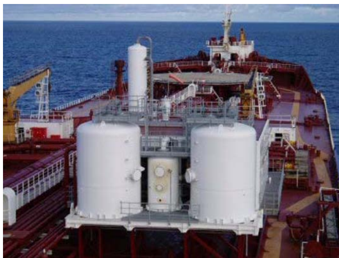
Figure 5-8. Vapor Recovery Onboard a North Sea Shuttle Tanker
