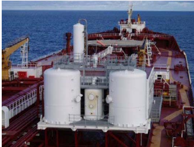
Figure 5-2. Vapor Recovery Onboard a North Sea Shuttle Tanker
